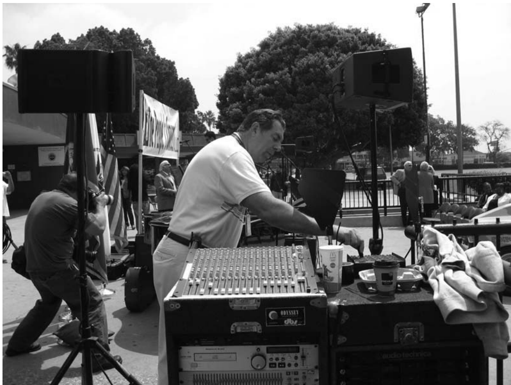
FIGURE 10.10 This reporter is plugging a portable Morantz recorder into a mixer. This mixer is used to amplify and combine the sounds from microphones picking up the announcer, singers, and musical instruments.
