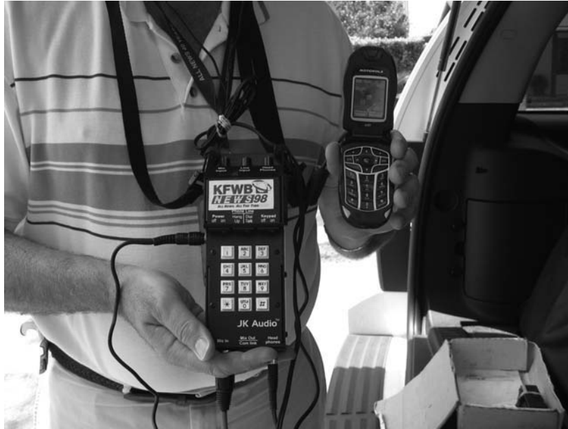
FIGURE 10.15 Equipment that can be used to send audio with a cell phone.
