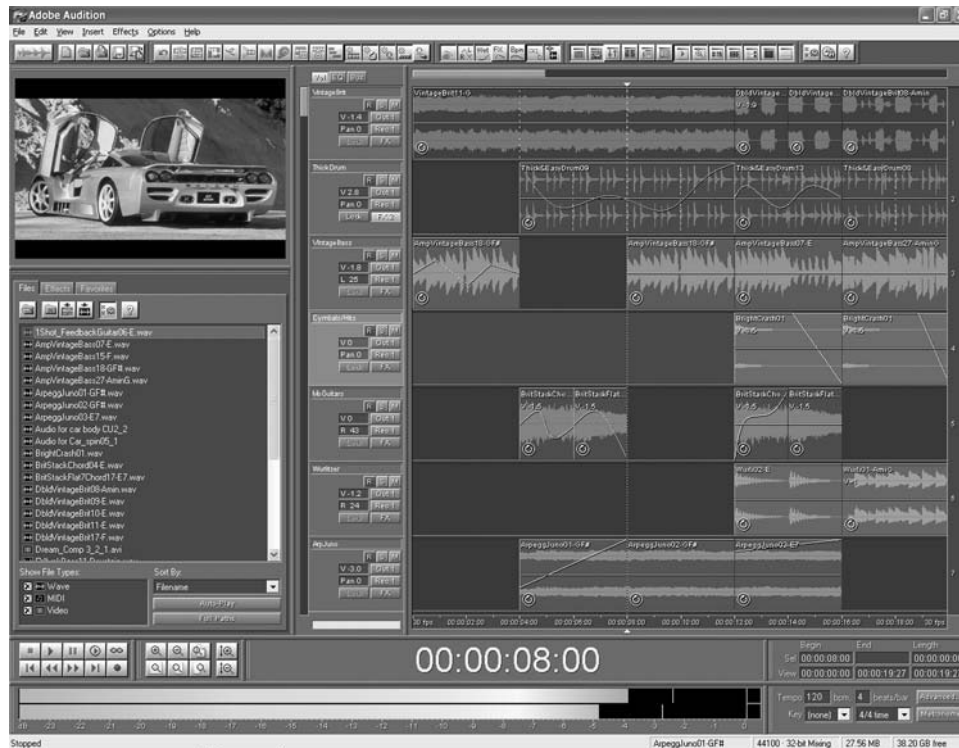
FIGURE 3.10 Most digital audio editing programs incorporate a virtual multitrack recorder. (Adobe screenshot reprinted with permission from Adobe Systems Incorporated.)
