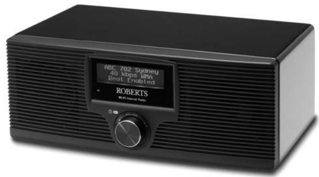
FIGURE 12.4 This Wi-Fi radio and media player can receive Internet radio stations, podcasts, and other audio streams, as well as streaming music stored on your PC through the radio. (Image courtesy of Roberts Radio.)
