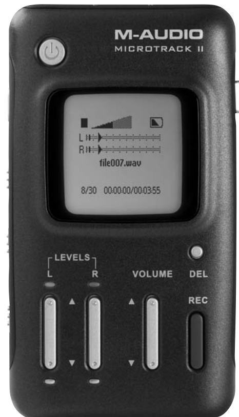
FIGURE 6.10 Many solid-state digital audio recorders fit easily into the palm of your hand and have become popular for news gathering and other field recording uses. (Image courtesy of M-Audio.)
