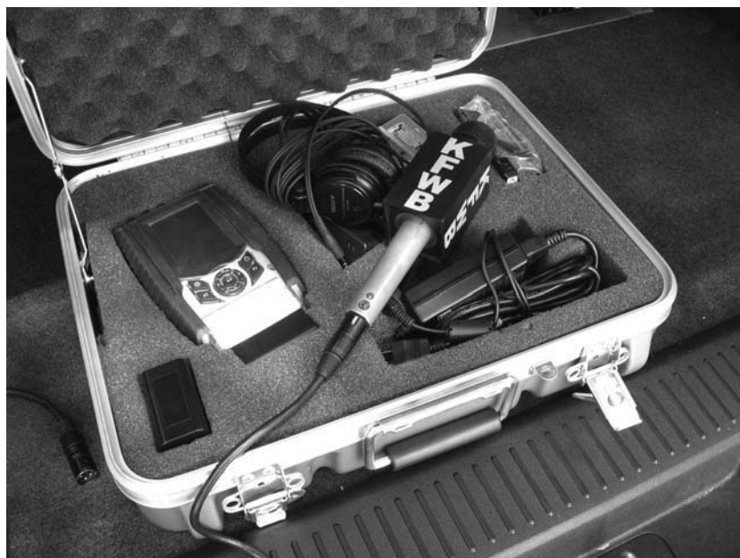
FIGURE 10.14 Equipment needed for wireless broadband transmission.
