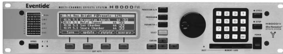
FIGURE 8.11 This multi-effects processor, an Eventide Harmonizer, puts several signal processing effects in a single “black box.” (Image courtesy of Eventide, Inc.)
