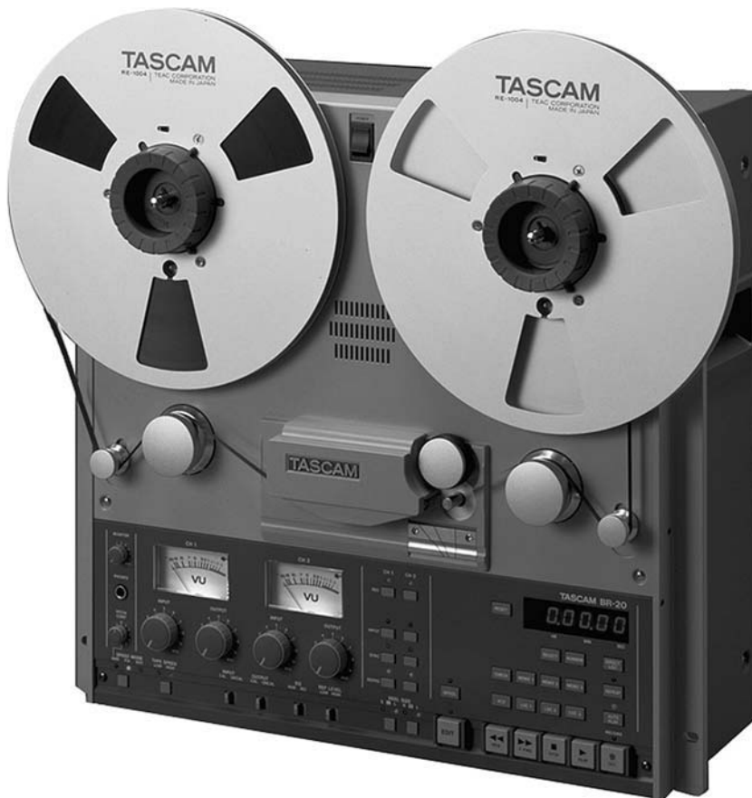
FIGURE A.4 The top part of this reel-to-reel recorder includes the supply and take-up reel, tension arm, tape guides, heads under the box with “Tascam” on it, capstan, pinch roller, and idler arm. The bottom section contains VU meters, pots, controls for playing, pausing, and so on, and various function switches to route the sound. (Image courtesy of Tascam.)
