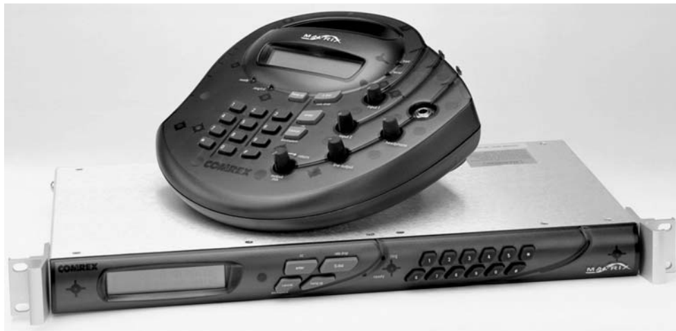
FIGURE 7.20 A telephone interface allows mixing an audio signal and a telephone signal. (Image courtesy of Comrex Corporation.)
