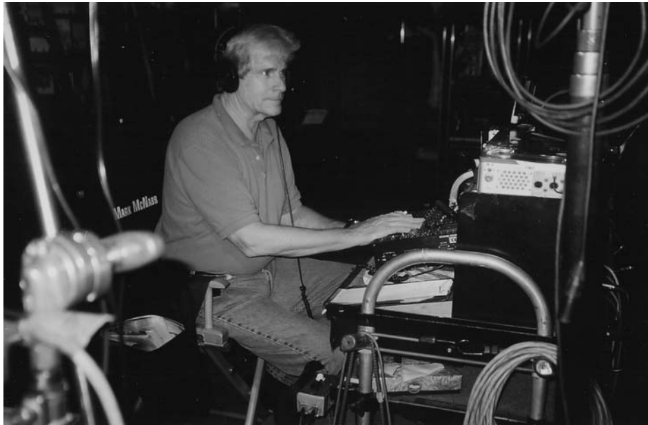
FIGURE 11.7 This audio operator is sitting in a corner of a studio where a scene for the TV show Family Affair is being shot. He has all his equipment on a portable cart.
