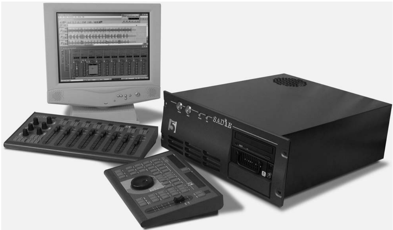
FIGURE 3.4 Some digital audio workstations resemble desktop audio editors, but employ specialized audio cards, customized boxes, and proprietary software. (Image courtesy of SADiE Inc.)
