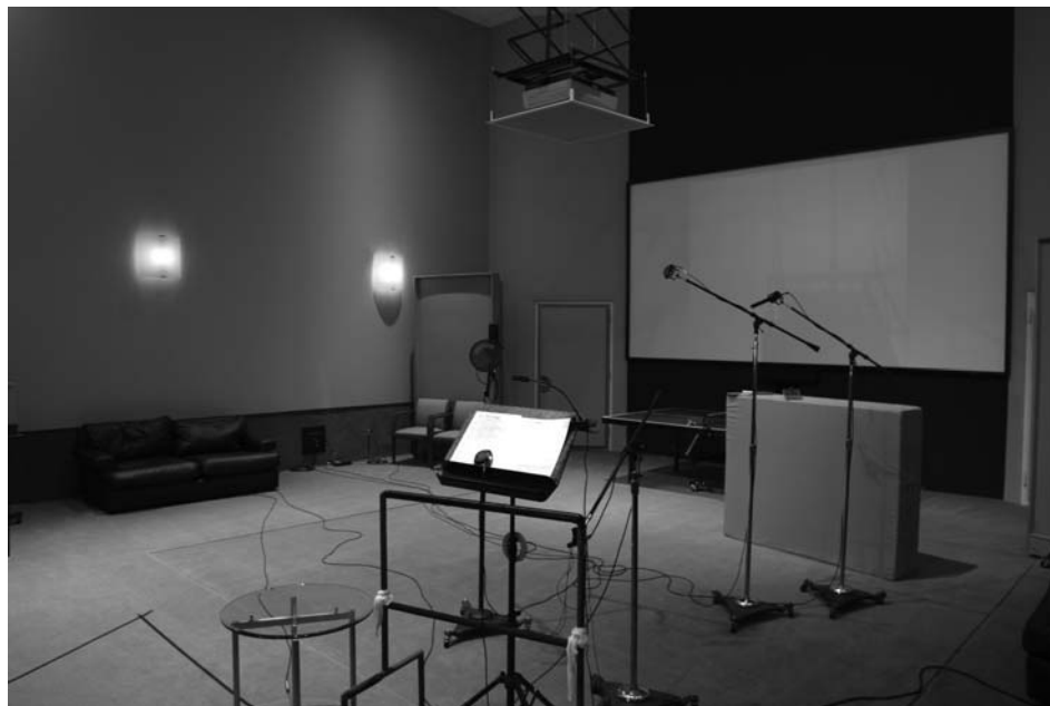
FIGURE 11.11 An ADR facility. Actors undertaking ADR look at the screen to sync the sound. They can stand or sit on the stool and that way they can move if they need to change perspective. Having a podium where they can place a script or notes also helps the process. (Image courtesy of Sony Pictures Entertainment.)
