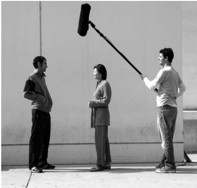
FIGURE 11.1 A boom operator (right) readying a fishpole for use. It is best to position the fishpole so the mic is 1 to 4 feet in front of the mouth of the person speaking and 1 to 3 feet above it.
