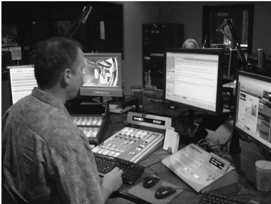
FIGURE 9.5 This setup at an all-news stations is made for two anchors. Each has his/her own audio board, monitors, and other equipment. By positioning their monitors appropriately, they are able to maintain eye contact.
