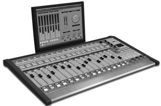
FIGURE 5.4 Many digital audio consoles are merely control surfaces that work in conjunction with a separate audio router that allows the electronics to be centralized in a rack or equipment room. (Image courtesy of Wheatstone Corporation.)
