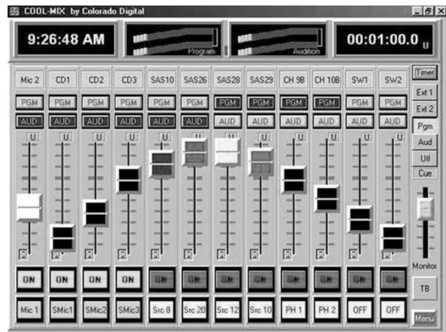
FIGURE 5.5 “Virtual” audio console controls emulate the functions of the traditional audio board. (Image courtesy of Arrakis Systems, Inc.)
