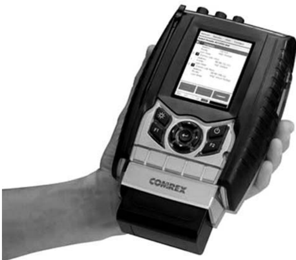
FIGURE 7.21 This portable IP audio codec can interface with DSL, cable, Wi-Fi, 3G cellular, satellite, POTS, and other communication services. (Image courtesy of Comrex Corporation.)
