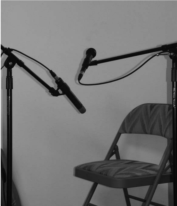
FIGURE 9.4 This is an effective setup for a person who plays guitar and sings. One mic is by the person’s mouth and the other is by the guitar sound hole.
