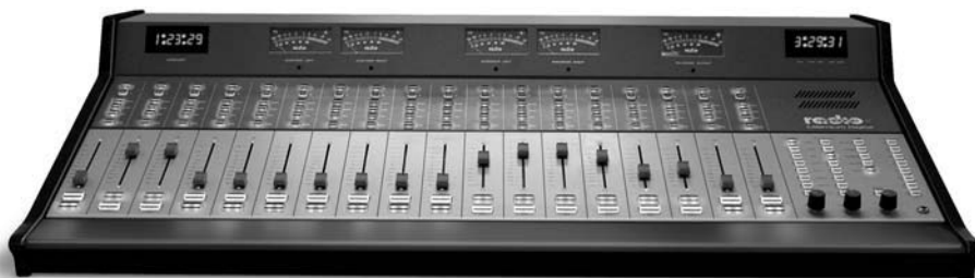
FIGURE 5.2 Some digital audio consoles feature a self-contained, modular architecture, much like older analog boards. (Image courtesy of Radio Systems.)
