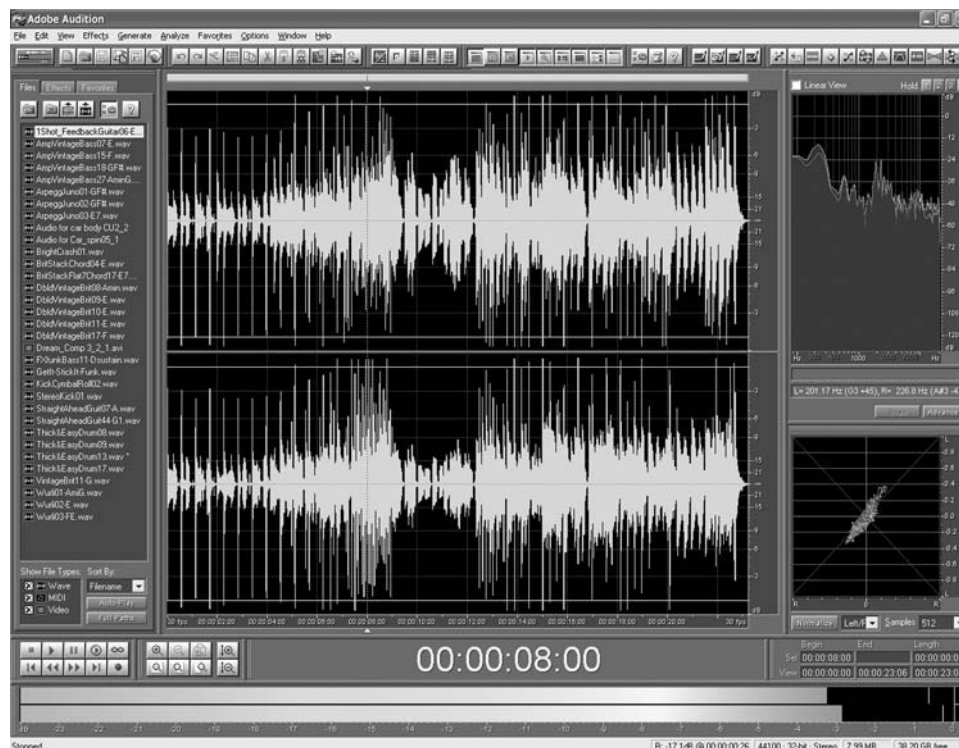
FIGURE 3.8 The main screen of an audio editing program shows various navigation and functional controls for manipulating the audio file. (Adobe screenshot reprinted with permission from Adobe Systems Incorporated.)
